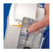
Grasp thumb tab on valve and insert ring retainer directly into left pocket. Press down on thumb tab to ensure valve is fully seated. Thumb tab must align with white line on left.
